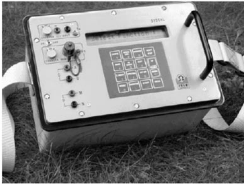
Figure 2. The SYSCAL Junior made by IRIS INSTRUMENTS Ltd. for RIP
